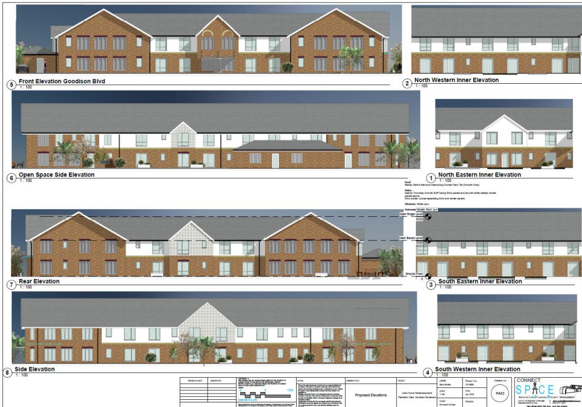
Fig 6: Showing the proposed elevations with a simpler roof design, which has the benefit of reducing the scale of the building.
