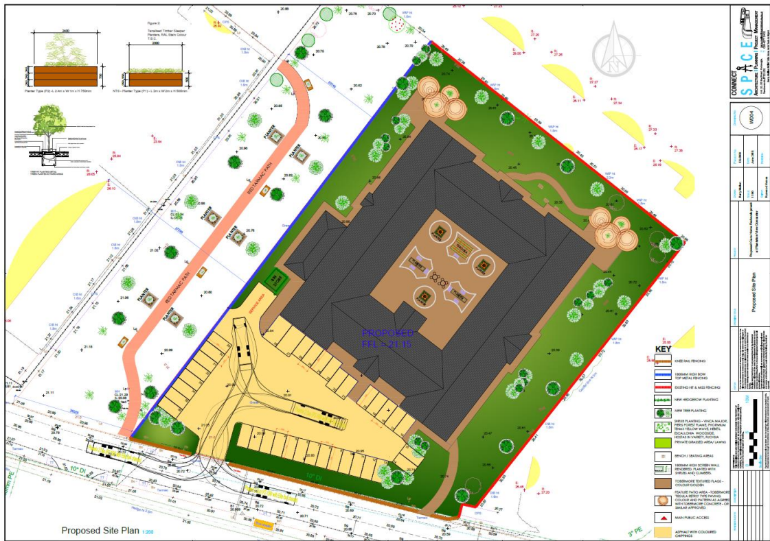
Fig 2: Showing the proposed site layout for a 83 bed care home, which is in the same position and has the same footprint as the original approval.
